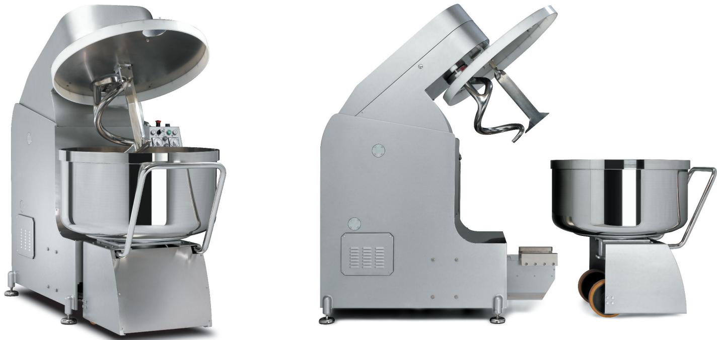
The new taper bowl locking and motion system is technically superior to the traditional systems as it utilizes a taper coupling to join the machine and the trolley. The trolley is locked by means of a taper shaft that, as it ascends, centres the bowl and moves it into the working position.
